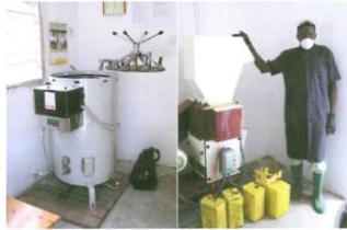
Figure 14: Example of autoclaving and shredding in Tanzania
