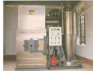
Figure 12: Example of dual-chamber incinerator for healthcare waste treatment
